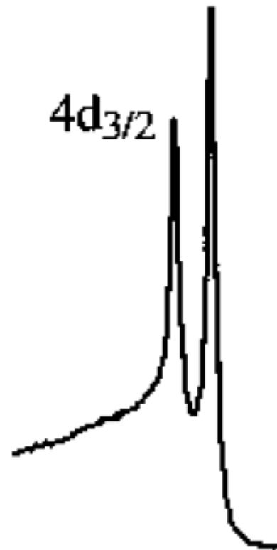
The separation between the two peaks are named **spin orbital splitting**. The values of spin orbital splitting of a core level of an element in different compounds are nearly the same.
