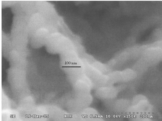
Fig. 1. SEM image of the fresh nanoscale iron particles.
